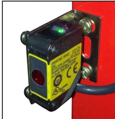
Power on & not aligned
